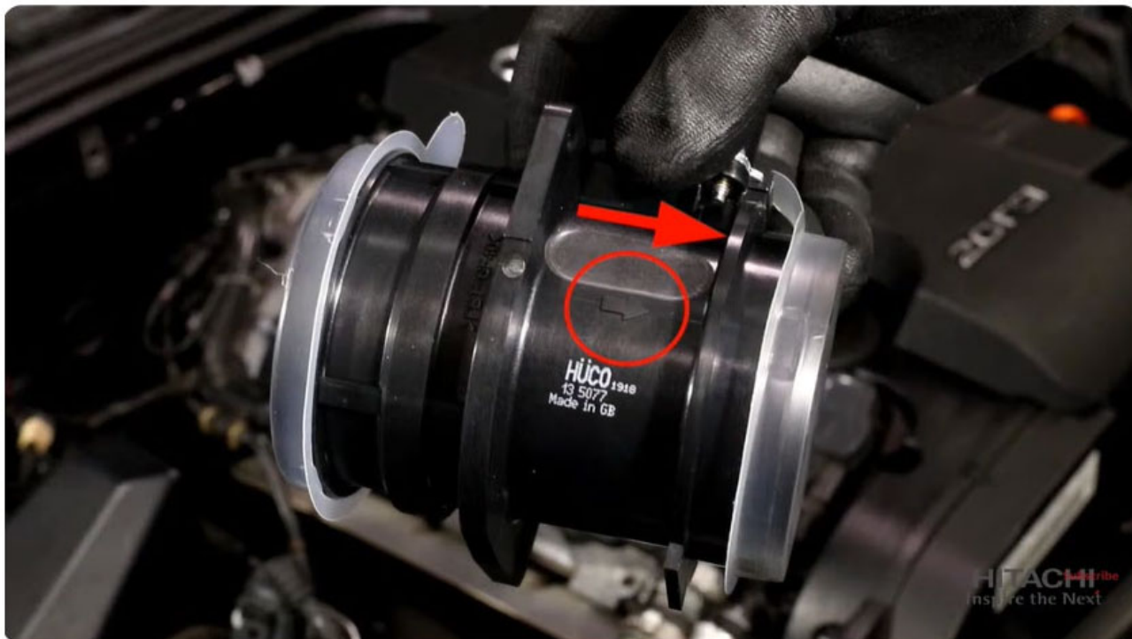
Air flow sensor EASY replacement on TFSI engine | Astemo Aftermarket Germany
